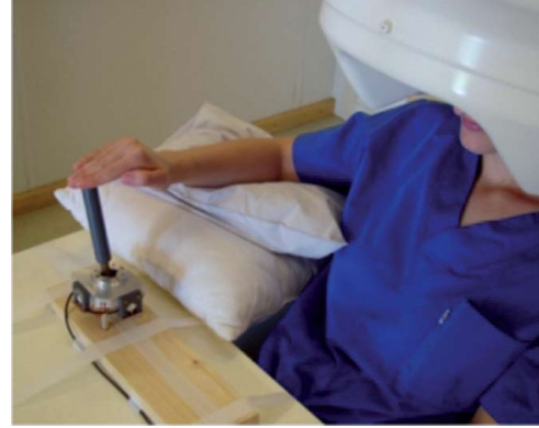
The subject is moving a joystick in one of four directions, while brain activity is recorded by MEG (sensors under the white cap) and EEG (not visible in this figure).
