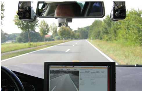
Driver assistance system DRIVSCO: Screen for monitoring the course of the road.
